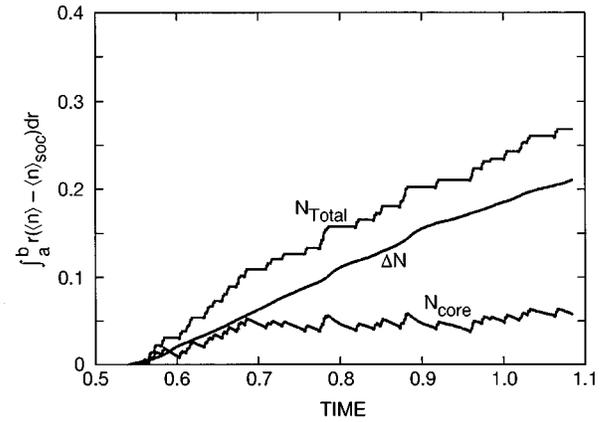
FIG. 3. Time evolution of the total pressure and the pressure in the core. The system reaches a steady state when  $N_{\text{core}}$  stays constant in time.
