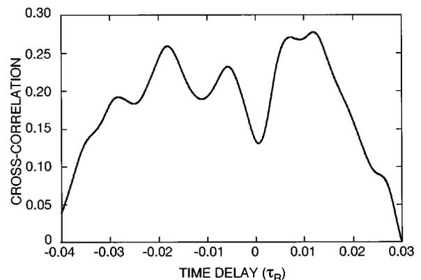
FIG. 16. Cross-correlation of the low frequency modulation at  $r/a=0.35$ . The cross-correlation has a double peak at  $\pm \Delta t$ , the time delay corresponding to the propagation distance of the avalanche.
