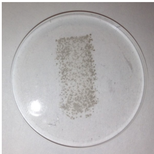
Figure 4.19 Burn marks on the excimer laser rear mirror after several nights of operation.
