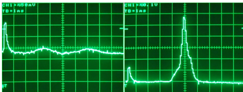
Figure 2.9 Spectra of Na emission and the dye laser beam through a high-resolution spectrometer. Na D 2 and D 1 lines from an Na lamp (left); the laser line through the same spectrometer when centered on the D 2 line (previously aligned with the center line on the oscilloscope display). The display scale in the horizontal is 1 ms on both plots and in the vertical is 50 mV (left) and 100 mV (right).
